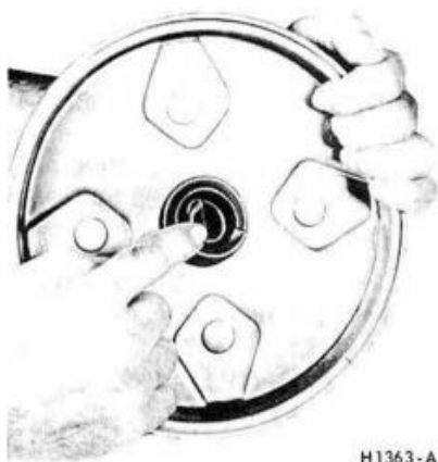
FIG. 44—Removing or Installing Rear Seal to End Plate—Midland-Ross
