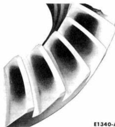
FIG. 7—Acceptable Non-Hunting Gear Set—Coast Pattern
