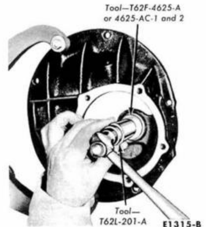
FIG. 41—Installing Pilot Bearing
