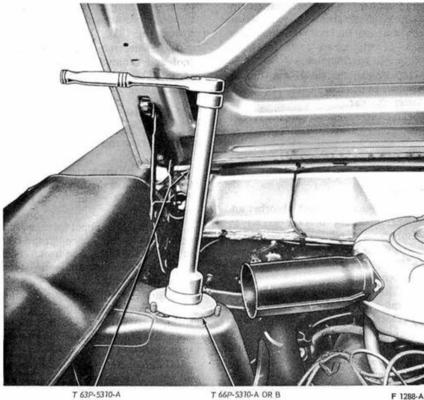
FIG. 12—Spring Compressor Installed—Upper View—Comet, Falcon and Fairlane
