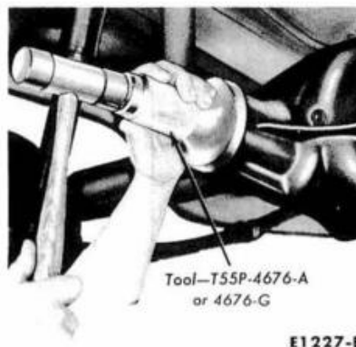
FIG. 12—Typical Drive Pinion Flange Seal Installation
