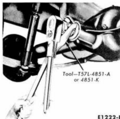
FIG. 10—Typical Drive Pinion Shaft Nut Removal
