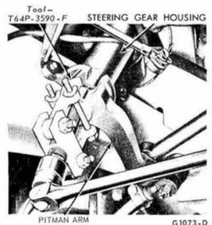
FIG. 7—Removing Pitman Arm—Typical
