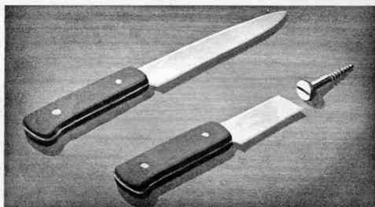
SCREWDRIVER MADE FROM KNIFE
