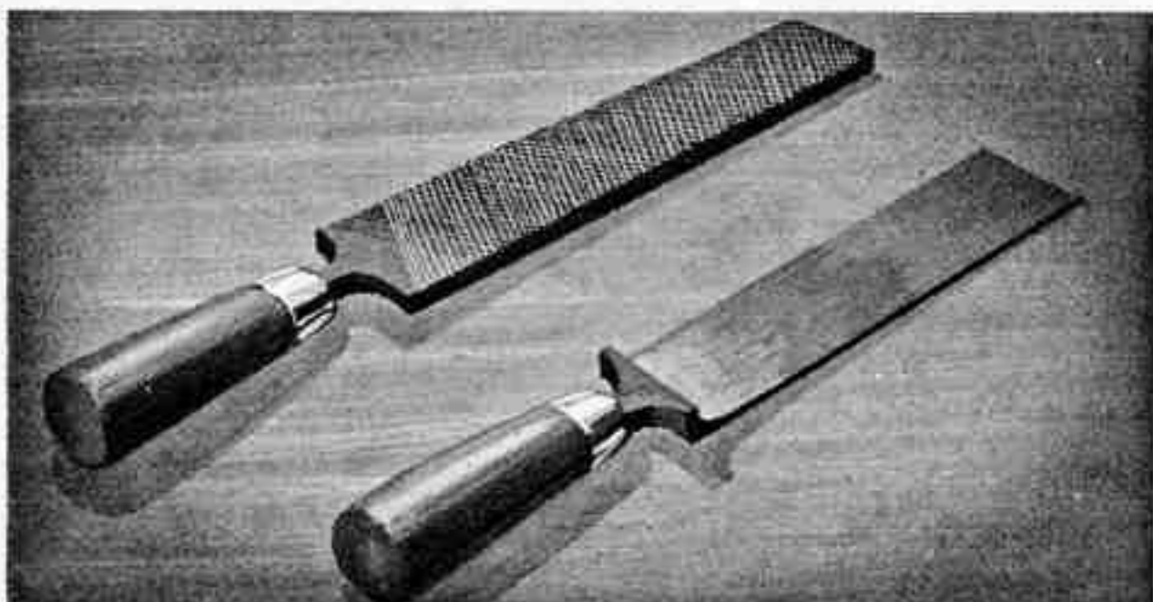
SCRAPER MADE FROM FILE
